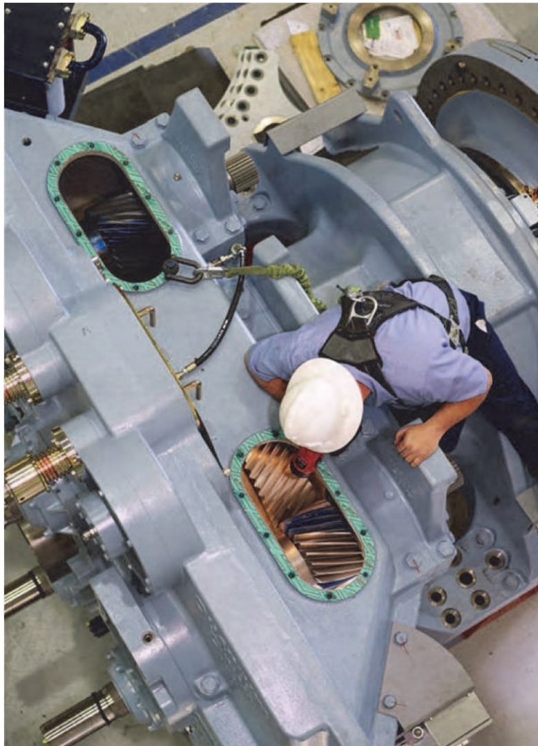
Figure 3.8: Top view of a Liberty Quantum Drive 2.5 MW rated power wind turbine gearbox.
