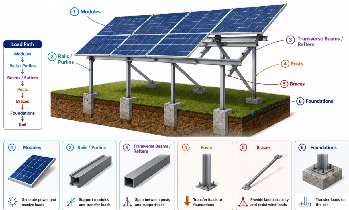
Figure 3.4: Ground-mounted PV structure components breakdown.
