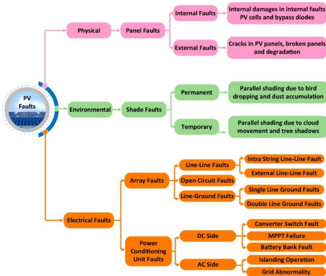
Figure 4.10: Three fundamental categories faults in PV
