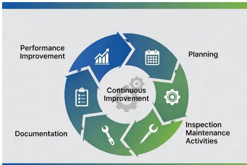
Figure 3.1 Preventive Maintenance Cycle
