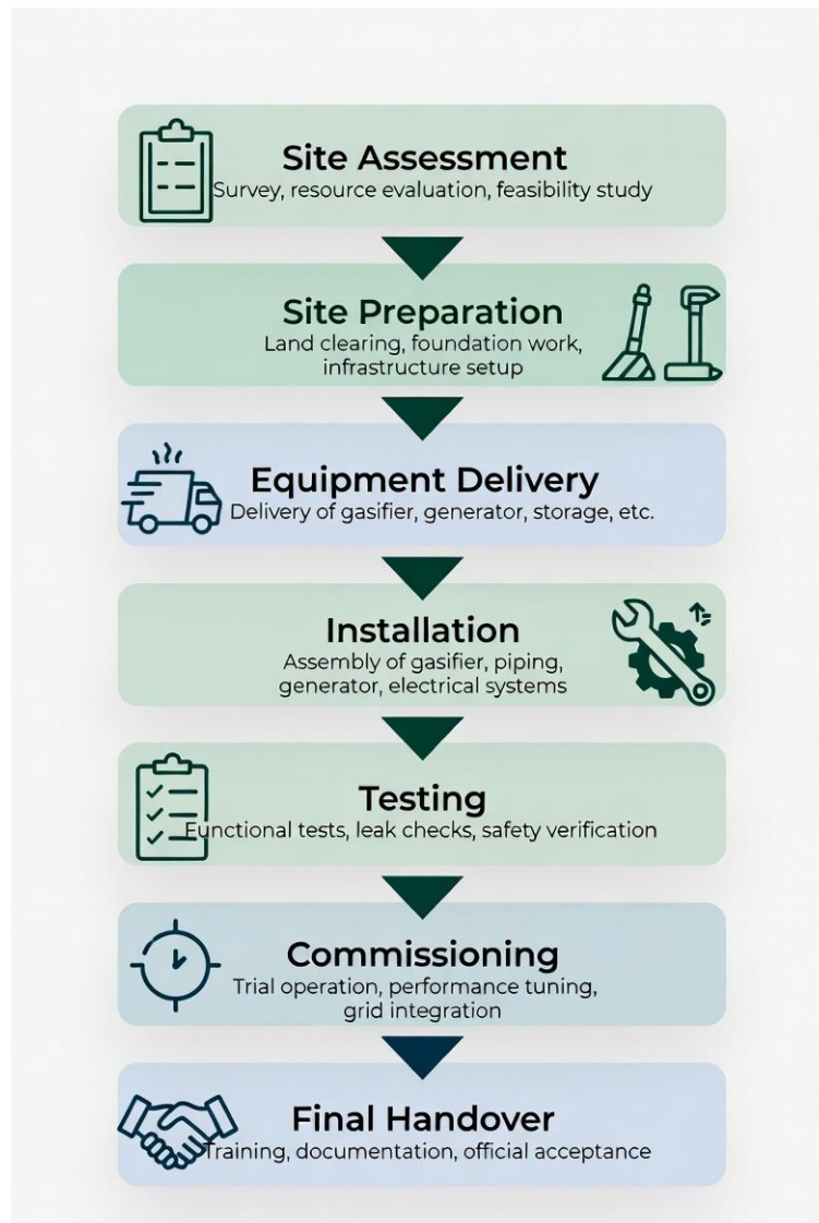
Figure 1.1: Biomass Energy System Installation Process
